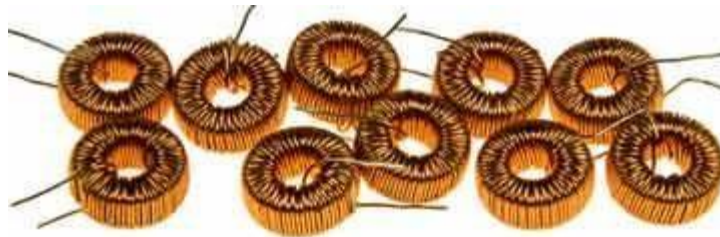
Inductors on a toroidal ferrite former
